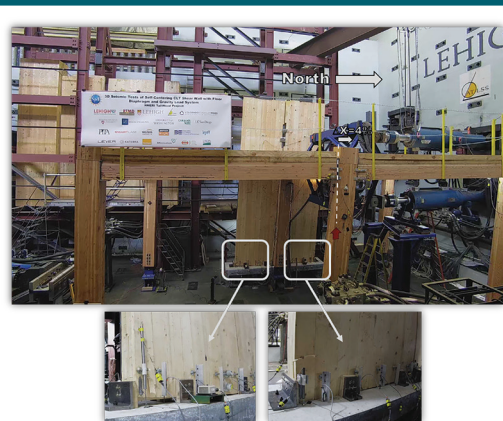
Test sub-assembly under bidirectional loading
