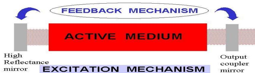
Figure 2.2. Laser components
