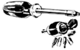
**Interchangeable Magnetic Tip Screwdrivers.** These screwdrivers have a magnet in the shaft so that they not only hold the bit but can also hold the screw. In addition, the variety of bits for this type of screwdriver is limitless and the unused bits can be stored in the handy compartmented handle.
