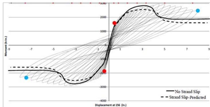
Figure 2: Single Pile Test Data (Moment-Displacement Curve).
