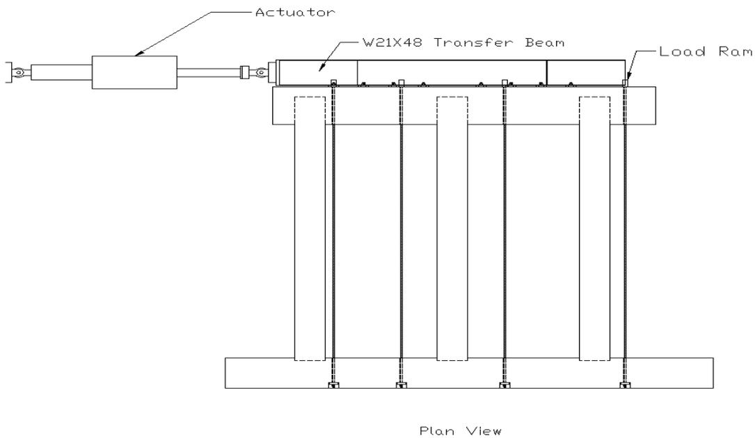
Figure 3: 3-Column Bent Test Setup
