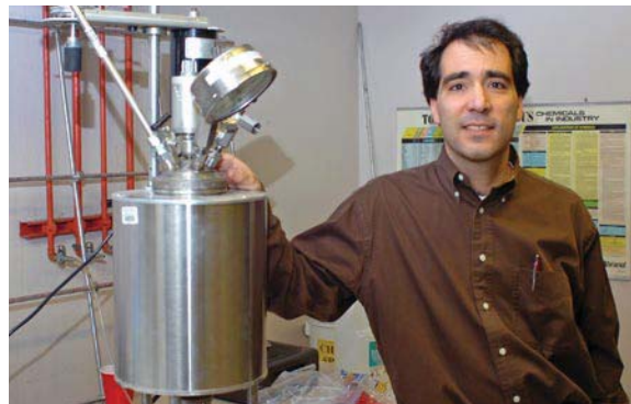
Professor Charles Coronella with equipment that subjects biomass to 3,000 psi of pressure as part of the conversion process.
