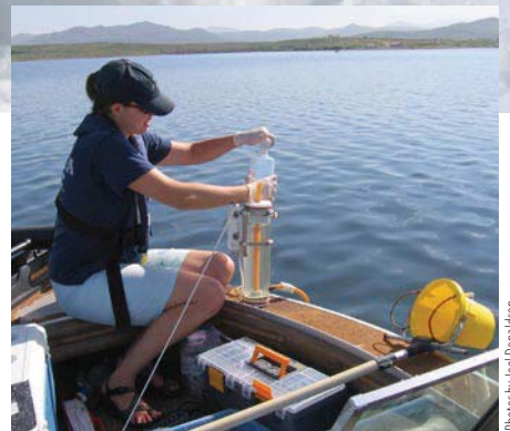
TOP: Graduate student Melissa Markee, 26, measures the pH of the water at Wild Horse Reservoir during the winter. INSET: Markee collects water samples during the summer from Wild Horse Reservoir using a Van Doren sampler.
