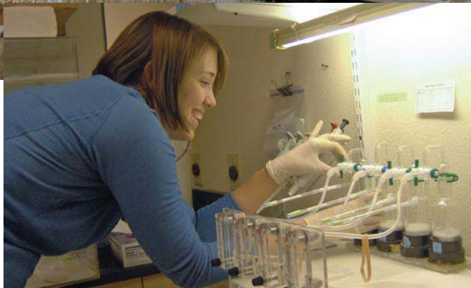
TOP: The Ruby Marshes have a desolate beauty all their own during the winter. LEFT: Markee turns the air flow on to bubble reservoir water samples onto traps to test for methyl mercury. RIGHT: Cooperative Extension faculty Sue Donaldson (left) and Kerry Seymour discuss the results of a survey of licensed fishermen to determine their fish-consumption habits.
