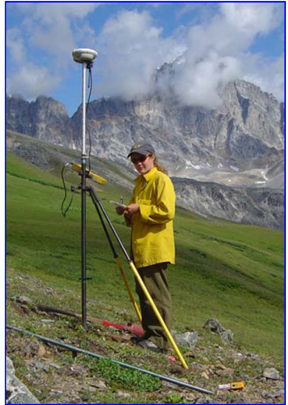
Hansen used GPS to record an exact location for setting up a surveying monument on Revelation Mountain, AK.
