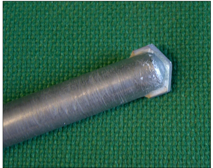
Figure 1. Tungsten carbide hammer drill insert silver-soldered on tip of 1/4" schedule 40 steel pipe probe. This design was abandoned in favor of the model shown in Figure 2.
