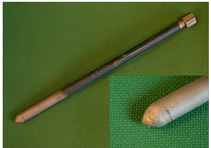
Figure 2. Final probe design with hard-faced tip and hex cap on top end of 1/4" schedule 80 seamless steel pipe. Close up shows tungsten carbide particle-containing hard-faced tip. (Note probe shown is 12" long for illustration purposes.)
