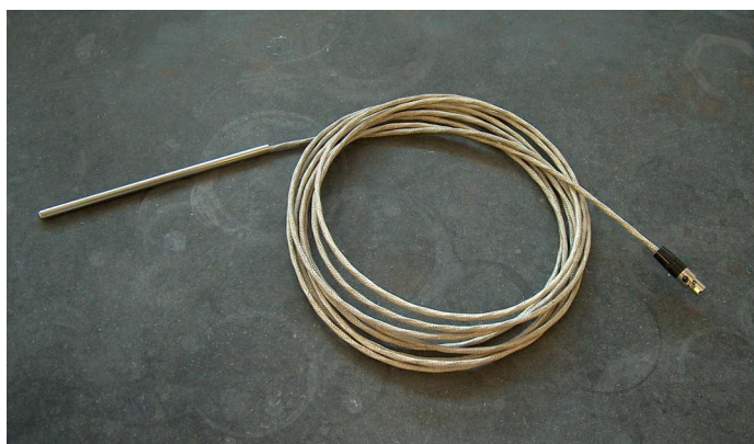
Figure 3. RTD sensor potted in \frac{1}{4} " stainless tube with 4 wire cable and miniature connector.
