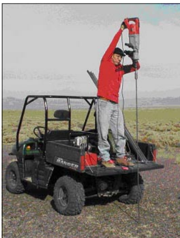
Figure 5. 1/4" steel pipe probe being driven into ground with electric demolition hammer, and complete field setup of utility vehicle with approximately 20 2.2m probes, demolition hammer, generator. (From Coolbaugh et al., 2007).
