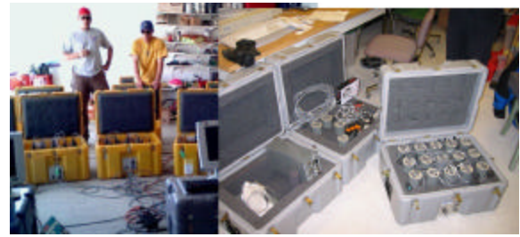
Figure 5: Compact 20-channel Reftek RT-125 “Texan” crustal refraction recording system acquired under the previous year of this project (front). 199 Texans owned by the NSF during deployment on the No. Walker Lane Refraction Survey, May 2002 (back).
