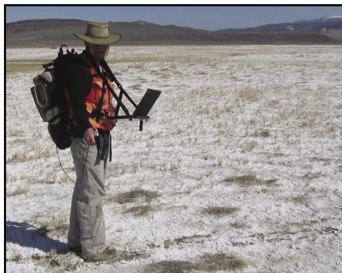
Figure 2. ASD spectroradiometer deployed at Salt Wells. Tincalconite and halite both appear in the photo as efflorescent evaporite crusts.
